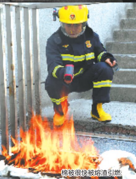
掉落的熔渣瞬间引燃海绵
